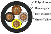
Polychloroprene rubber outer jacket Bare copper conductor EPR insulation Green/Yellow wire
